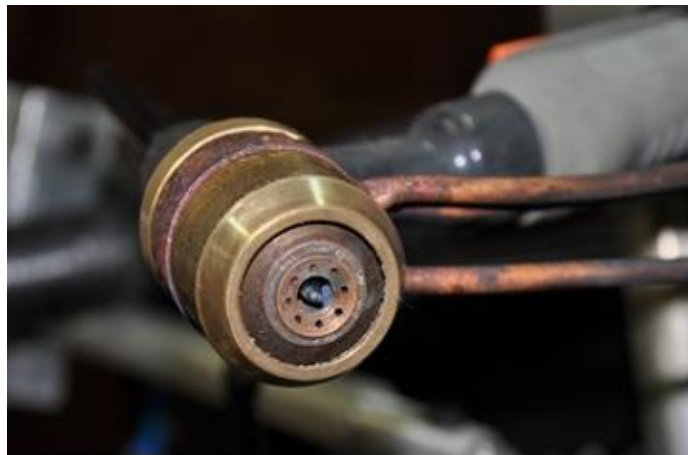
Figure 3. Photo of the bottom view of the torch adapted test after deposition.
